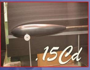
Tested in the UT Wind Tunnel with a measured drag coefficient of .15 Cd
