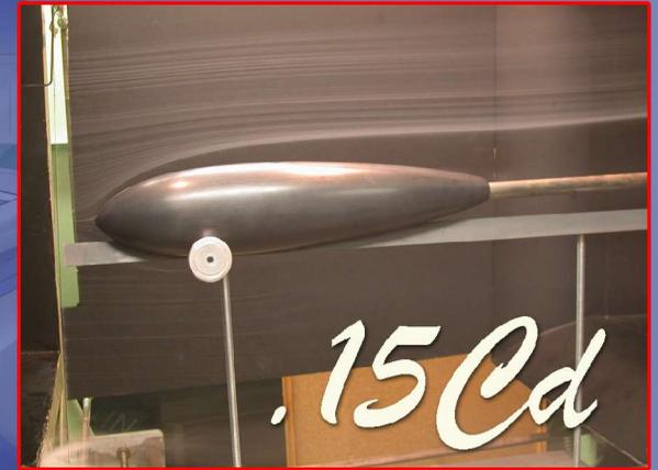
Tested in the UT Wind Tunnel with a measured drag coefficient of .15 Cd
